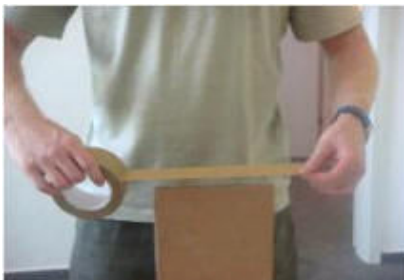
1. Hold the cut edge upwards. Roll out the tape with a 3 to 5cm overhang at each side.
